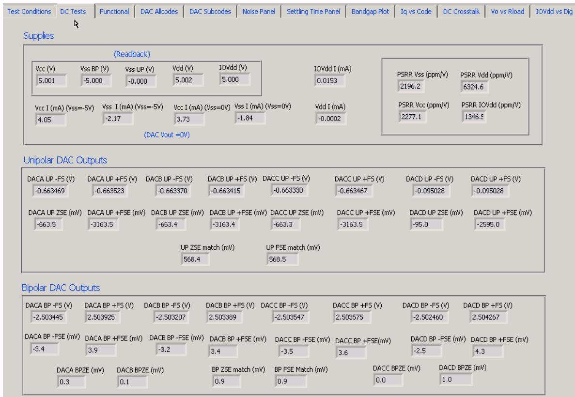
Figure 2–8. DAC7654 EVM Test Parameters and Results in Bipolar Configuration
